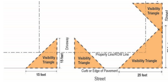
Figure 106.86-1 Visibility Triangles at Driveways and Intersections
