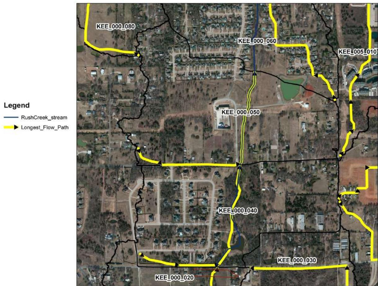
Figure 2-3. Longest flow paths for subbasins at the Kee branch Headwaters.
