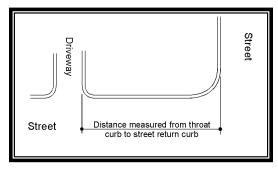
flow and safety characteristics of the driveway and public street. The distance will be measured from the nearest edge of the driveway return to the intersecting street curb return.
